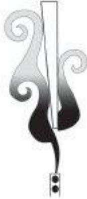
Fig. 45 – Effect of flute on the surrounding air
