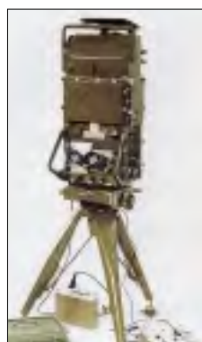
ЛЦД-1Д22 1D22 laser ranger designator
