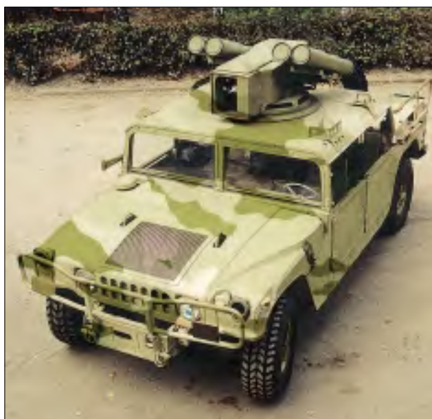
Kornet-E ATGM system with 9P163-2 launcher mounted on Hummer motor vehicle
