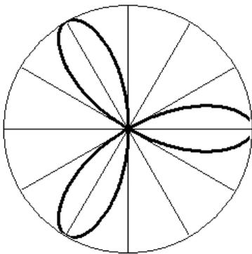
$$\begin{aligned} S &= 6 \cdot \int_0^{\pi/6} \frac{1}{2} a^2 \cos^2 3\varphi d\varphi = \\ &= 3a^2 \int_0^{\pi/6} \frac{1 + \cos 6\varphi}{2} d\varphi = \frac{3a^2}{2} \left( \varphi + \frac{1}{6} \sin 6\varphi \right) \Big|_0^{\pi/6} = \\ &= \frac{3a^2}{2} \left( \frac{\pi}{6} + \frac{1}{6} \sin \pi - 0 - \frac{1}{6} \sin 0 \right) = \frac{\pi a^2}{4}. \end{aligned}$$
