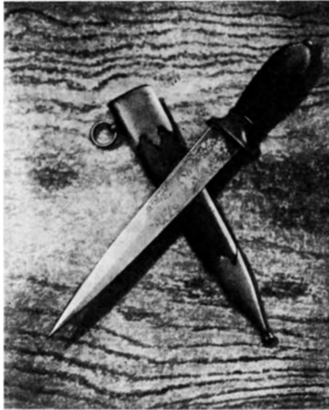
Fig. 11—Damascus steel dagger. The background is a photograph of the etched damask pattern of the blade, magnified 8 times (Ziegler, Mining and Metallurgy , v. 20, 1939, p. 69).
