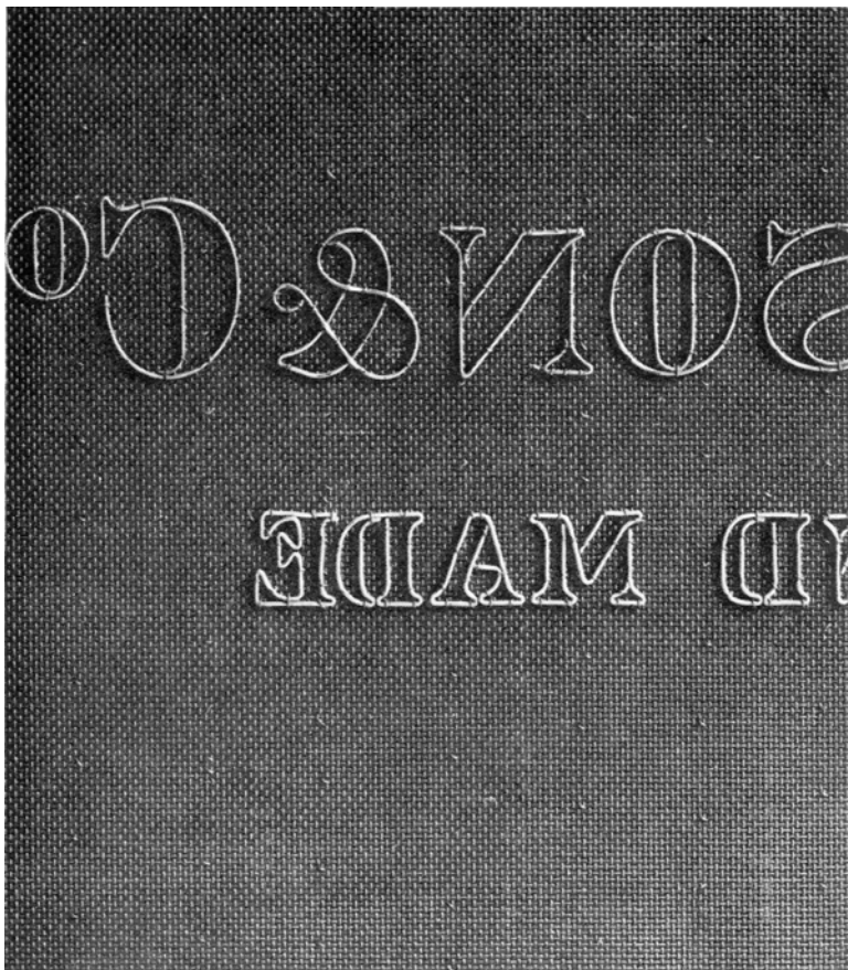
Сетка Ватмана [ Hunter D. Papermaking. The history and technique of an ancient craft. London: Pleiades Books, 1947. С. 126, рис. 101 ]
